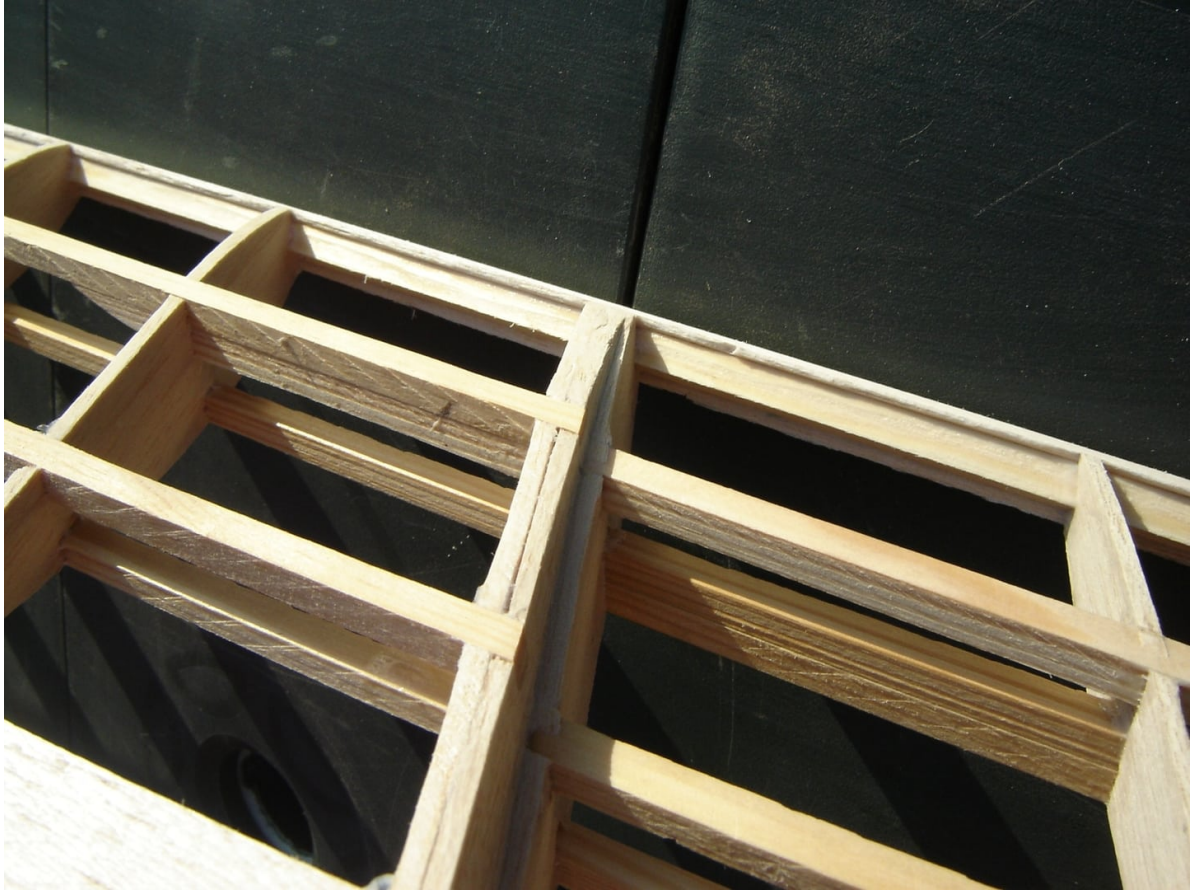
Construction where the wing tip is attached to the main wing section.
